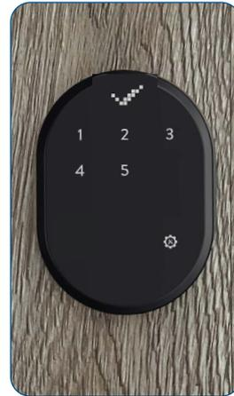
When the confirmation symbol appears on the display, all user passwords have been successfully deleted (except the master password). The device will then switch off
