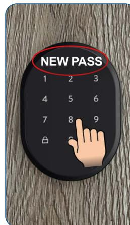
NEW PASS appears in the display. Type in your new 5-digit master password for the first time, which will then appear again in the display
