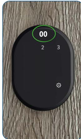
The number 00 appears on the display. Only the numbers to which a password has been assigned (in this case 02 and 03) light up on the keypad. The 01 is assigned as the master password and cannot be deleted. Therefore the 1 is not illuminated
