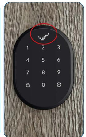
The display shows the OK sign (check mark) and then 01. Your master password has been successfully created. The device will then switch off
