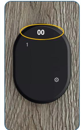
The display shows 00. Only the number 1 and the menu key light up on the radio keypad
