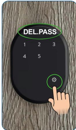
DEL.PASS (=delete password) appears on the display. Confirm by clicking on the right menu key or setting key
