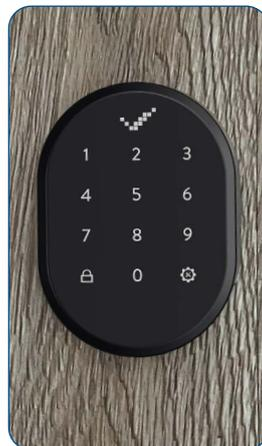
The Smartlock ÜTOPIC emits a short warning tone and couples the wireless keypad with the motor cylinder. The OK sign appears in the display
