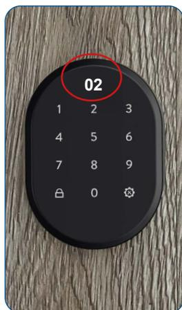
The display shows the number assigned by the device under which the user password (02-06) was stored. Then the wireless keypad switches off
