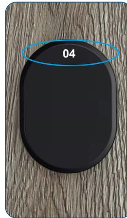
The display shows the number of assigned passwords,... e.g. 04 (a total of 4 passwords have been created here). The wireless keypad will then switch off
