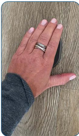
Wake up the device by placing the palm of your hand on the surface of the wireless keypad
