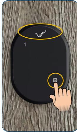
Touch the right menu key or setting key until the OK sign (check mark) appears in the display. The wireless keypad then switches off. The device was successfully reset
