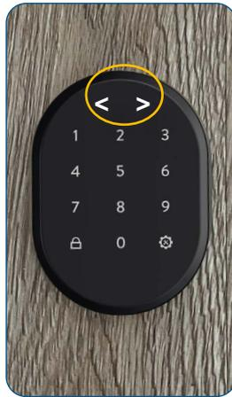
The LED indicator is activated and two arrows pointing in opposite directions < > appear in the display
