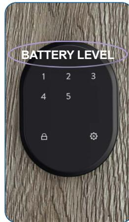
BATTERY LEVEL (=battery status) appears in the display
