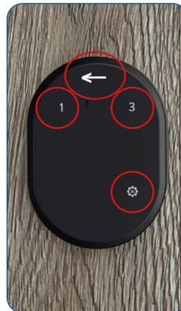
Only keys 1, 3 and the right menu key or setting key light up. The arrow in the display moves alternately to the right and left
