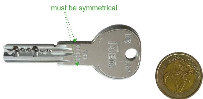
The thickness of the key should be at least 2.4 mm wide. If it is thinner, then wrap several times with adhesive tape until a thickness of approx. 2.4 mm is reached! A 2 euro coin has the ideal thickness - therefore it is best to use it as an aid.
