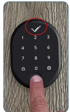
Place the master fingerprint on the sensor or type in the 5-digit master password until the OK sign (check mark) appears in the display
