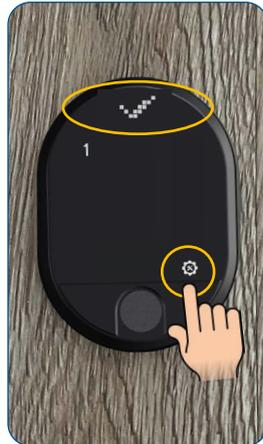
Touch the right menu key or settings key until the OK sign (check mark) appears in the display. The device has been reset successfully. The fingerprint reader with integrated keypad then switches off
