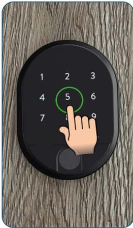
Touch the number assigned to the fingerprint from the device you want to delete (e.g. 5)
