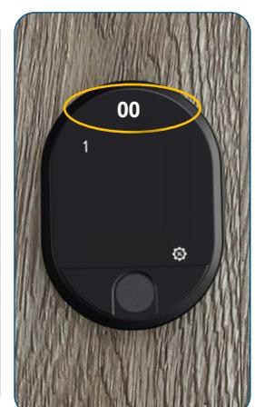
The display shows 00. Only the number 1 and the menu key light up on the device
