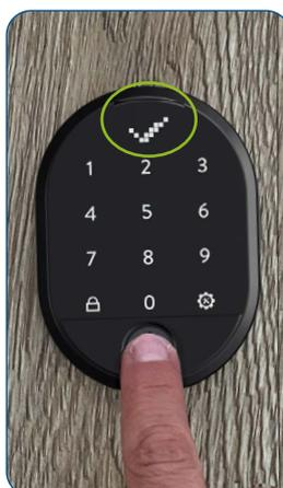
Place your finger on the sensor or type in the 5-digit password until the OK sign (check mark) appears in the display. The lock opens
