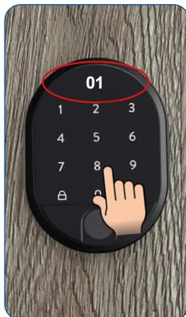
The number 01 appears on the display immediately afterwards. The master password was successfully changed at position 01. The device switches off automatically
