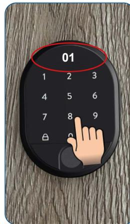
.... the number 01 appears on the display immediately afterwards. The master password was successfully stored at position 01. The device switches off
