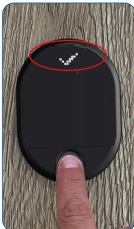
... the OK sign (check mark) appears in the display one last time. The fingerprint has been successfully stored. The device switches off
