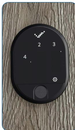
When the confirmation symbol appears in the display, the corresponding user password has been successfully deleted. The device then switches off
