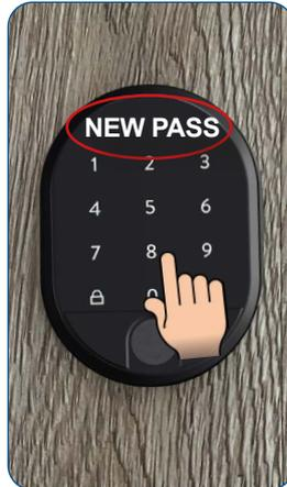
When NEW PASS (=New Password) is shown in the display type in your new 5-digit master password
