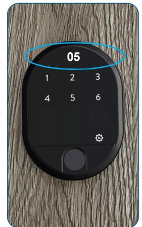
The number of assigned passwords appears in the display, e.g. 05. e.g. 05. The device then switches off
